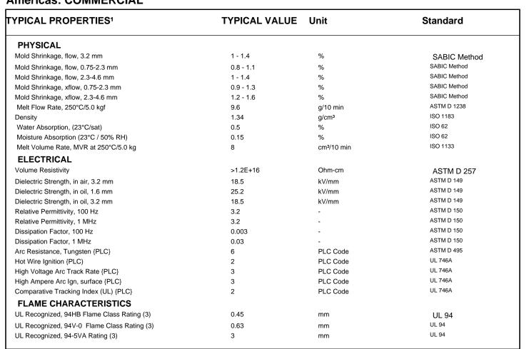
(1) Typical values only. Variations within normal tolerances are possible for various colors. All values are measured after at least 48 hours storage at 23°C/50% relative humidity. All properties, except the melt volume and melt flow rates, are measured on injection molded samples. All samples tested under ISO test standards are prepared according to ISO 294.
